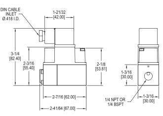
The Series 629HLP Differential Pressure Transmitters are suitable for measuring over-pressure, under-pressure, and differential pressure in compatible gases and liquids with 1% accuracy. The 629HLP is suitable for all measuring tasks in commercial, industrial or sanitary applications. Its single sensor design, allows it to measure small increment pressure changes, and converts them to a linear analog output signal from 4-20 mA or 0-10 VDC.
