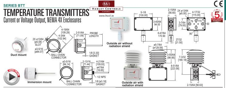
The Series BTT Temperature Transmitters offer transmitter output signals with the same form and fit as our popular TE thermistor and RTD sensors for building HVAC applications. Thermowells are required when using immersion models in liquid applications.
