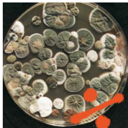
Sample from a compressor without dryer - moisture in the air provides ideal conditions for bacterial growth.
