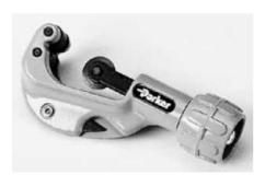
An adjustable tube cutter which produces a clean square end with no external burr and minimum internal burrs. The design of this cutter not only allows accurate positioning of the tubing onto the rollers but also allows the cutter wheel to be positioned both quickly and easily.
