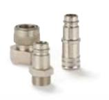
Brass coupling with no valve for applications with liquids in the pressure range up to 35 bar. The couplings are corrosion resistant. The system stands out for a high flow with minimal pressure drop.
