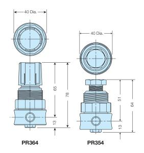
Note: 32mm dia. hole required for panel mounting.
