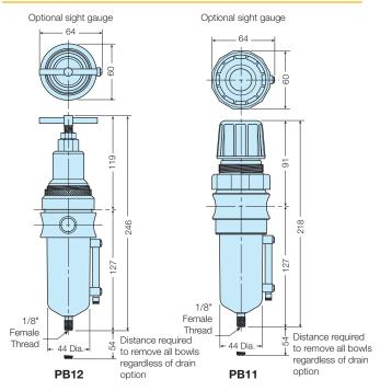
Note: 44mm dia. hole required for panel mounting.
