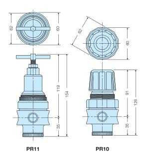
Note: 44mm dia. hole required for panel mounting.
