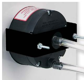
Mounting hardware is supplied with the MiniHelic® II gage for panel mounting through a single hole, 2-5/8" (67 mm) in diameter. Panel thickness up to 1/2" (13 mm) can be accommodated with the hardware supplied. If necessary, surface mounting of the gage can be accomplished by means of two 4-40 screws into the tapped mounting bracket stud holes in the rear of the gage. Surface mounting requires clearance holes in the panel for the two pressure taps.
