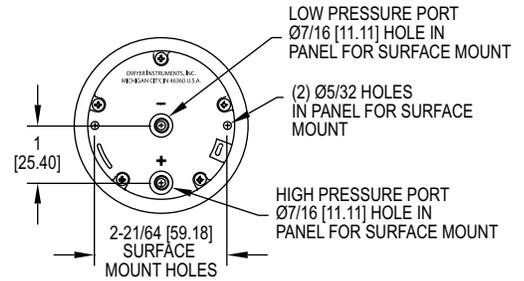
Combining clean design, small size and low cost with enough accuracy for all but the most demanding applications our **SERIES 2-5000** MiniHelic® II gage offers the latest in design features for a dial type differential pressure gage. It is our most compact gage but is easy to read and can safely operate at total pressures up to 30 psig.
