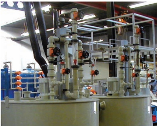
Chemical Conveyance in SYGEF Standard and Plus, PROGEF Standard and Plus, PVC-C, PVC-U, PE, CONTAIN-IT Plus
