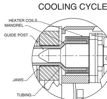
The tubing is inserted into the gun, and the jaws bite down on the tubing. The gun heats the tubing to the ideal temperature and alerts the user when the cycle is complete. At this time the flare mandrel is pushed into the tubing in the flare position where it is held for the cooling cycle
