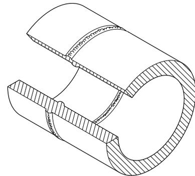
*Condition-* Bubbles in weld joint.
